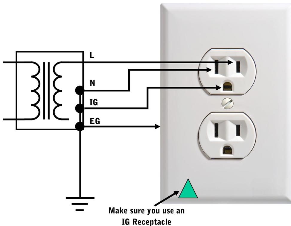
In theory, by not interconnecting this isolated ground to the equipment ground we can isolate stray currents and therefore voltages on the isolated ground. Remember IEEE deals not only with theory but actual application. When we look at what the IEEE has to say about isolated ground systems we get a better picture of their effectiveness.
