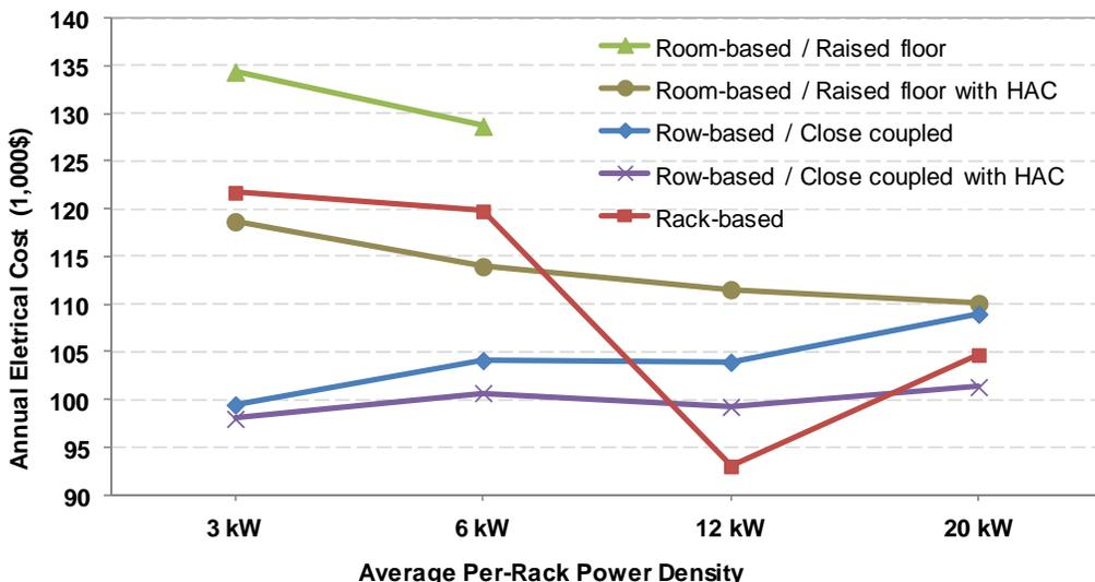
The electrical costs for room-based cooling without HAC are highest because the room-based cooling needs to move more air over larger distances and the CRAH units need to consume power to stir or mix the air within the room to prevent hotspots. This electrical cost is reduced by using HAC due to the separation of airflows. As density increases, energy costs decrease slightly due to the shorter pipe lengths and the associated decrease in pump power consumption.
