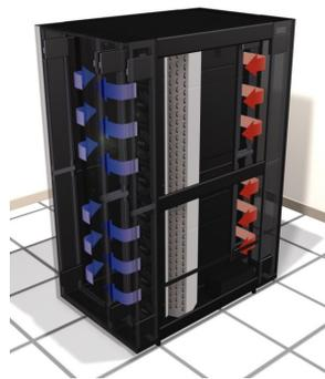
Similar to row-based cooling, rack-based cooling has other unique characteristics in addition to extreme density capability. The reduction in the airflow path length reduces the CRAH fan power required, increasing efficiency. As mentioned above, this is not a minor benefit considering that in many lightly loaded data centers the CRAH fan power losses alone exceed the total IT load power consumption.
